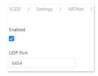
The gateway implements the Art-Net 4 protocol and can be used as a gateway by the main software and lighting control systems:
