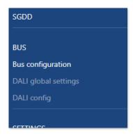
After enabling **DALI config** from the **Bus type** menu under **BUS 3** in **Bus configuration**, the configuration menu changes appearance, allowing addressing by **DALI config**, which takes the place of **DALI Controller** (required instead for communication with Control4).
