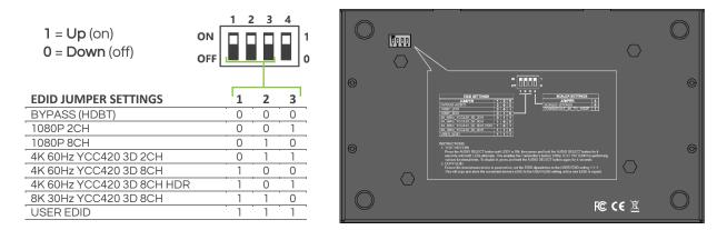
To copy the EDID from the connected device, ensure the downstream device is powered on, then set the EDID dipswitches to the USER EDID setting 111 (all up) on the Transmitter. This will copy and store the connected device's EDID to the USER EDID slot.
