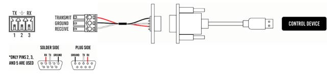
Wiring for this port uses a 3-pin terminal block connector to DB9 where only pins 2, 3, and 5 are used. If the devices do not have a DB9 port, a USB to DB9 adapter may be required.
