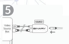
Insert one end of the multimode fiber cable with SC connector into the B10 extender labeled "source".
