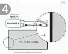
Connect the USB power and HDMI cables to the video source. Ensure the B10 extender labeled "Display" is connected to the video display.
