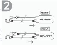
Insert USB power cable and up to 2 meter (6ft) B6 Premium High Speed HDMI Cable into each B10 Extender.
