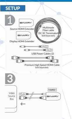
Connect the USB power and HDMI cables to the video source. Ensure the B10 extender labeled "source" is connected to the video source.
