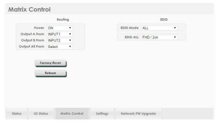
Any of the available inputs may be selected as a source for either of the two outputs by selecting the preferred input from the dropdown next to the "Output A" and "Output B" text.
