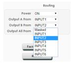
It is also possible to select a single source to be routed to both outputs quickly by selecting a source from the "Output All From" dropdown. Selecting "Masked" will output a blank video signal with no audio.
