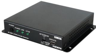
This HDMI Audio Extractor can extract up to 2 channels of LPCM audio or 5.1 channels of Bitstream audio from an HDMI source, allowing the user to convert high quality HDMI audio into more convenient analog (LPCM 2.0 sources only) or optical signals for use with powered speakers or non-HDMI AV receivers.
