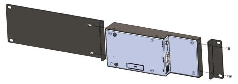
[Figure 2.5] Attaching brackets
