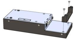
[Figure 2.4] Removing bracket
