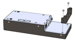
[Figure 2.7] Removing bracket
