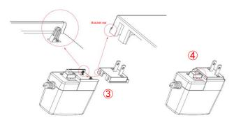
[Figure 6.2] Attaching AC plug
