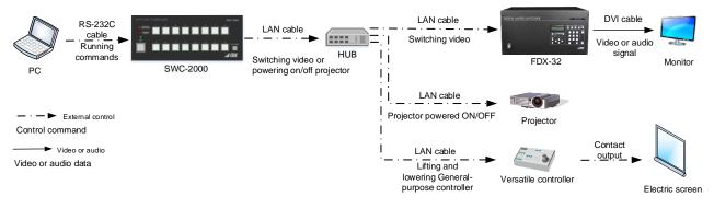
[Figure 3.2] System configuration
