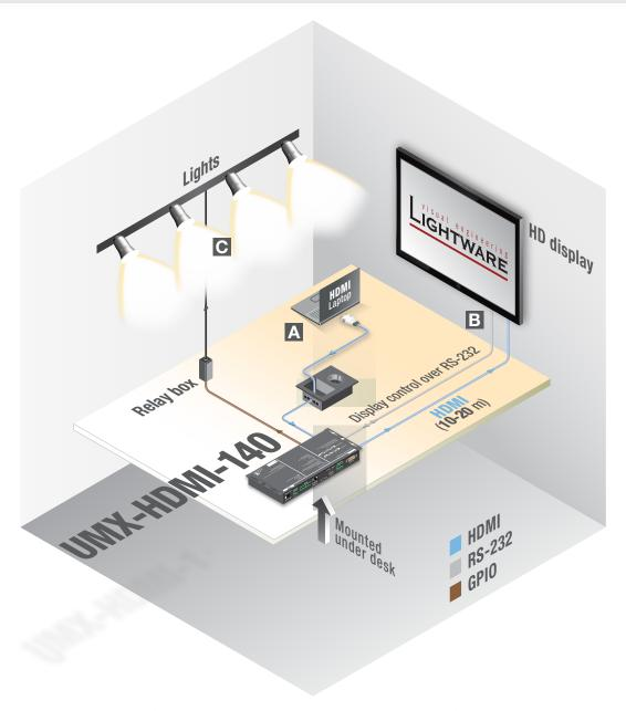
If a source is connected to the device, then the display turns on, the associated input will be switched to the output display and the lights turn on.
