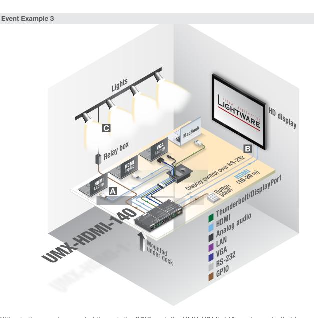
With a button panel connected through the GPIO port, the UMX-HDMI-140 can be controlled from a remote location. Input switching is available even if the transmitter is mounted under desk. In the example above there are three actions followed by a condition. When an input select button is pressed on the remote button panel, the selected input port is switched to the output, the display turns on, and the lights switch on.
