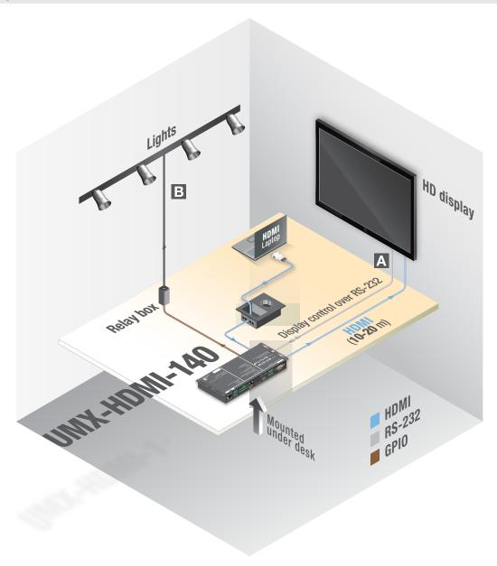
All sources are being disconnected from the switcher. The switcher is waiting for new input signal to appear. If no signal appears after a given time it switches the display and the lights off.
