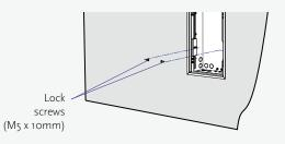
Once the frame is flush against the wall, lock it into place with the six M5 x 10mm button-head lock screws, and lock tight.
