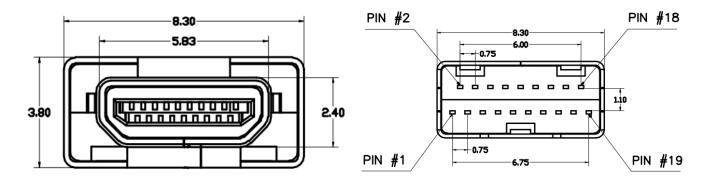
**HDMI** Type A /D Connector Pin Assignment
